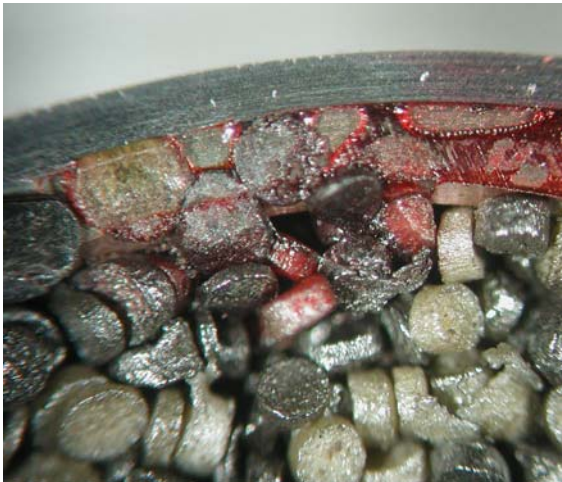
Figure 6 Red-dye leakage into pellet chamber
